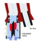
Shut off tools are equipped with an advanced silencer with a patented adjustable valve. During the rundown phase, the speed is decreased by means of a back pressure created by the adjustable valve. The slow run-down creates less energy and consequently improves the accuracy on hard joints at low torque levels.
