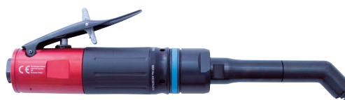
DR300-T...-T/S5-45 Series 300 W (0.4hp) / 550 to 5500 rpm
