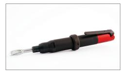
**TECHNICAL DATA WEN H04 Scaling Hammer** Air supply pressure 6 - 7 Bar Air consumption 200 litres/min Vibration level Below 3,8 m/s<sup>2</sup> (according to ISO 8662-2) Noise level (idle) 76 dB(A) Weight excl. chisel 1000 grams Length excl. chisel 255 mm Comes with a 15 x 100 tungsten carbide chisel
