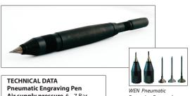
Air supply pressure 6 - 7 Bar Air consumption 15 litres/min Frequency 540 Hz Vibration level 1,6 m/s<sup>2</sup> Noise level (idle) 65 dB(A) Weight 150 grams **Size** 162 x 17 mm
