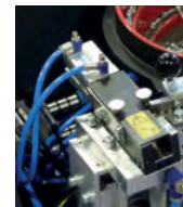
Escapement sensors Control/Secure escapement mechanism
