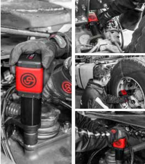
**Chicago Pneumatic** launches its first compact and robust pneumatic nutrunner, the CP66 series, perfect for flange-related and other bolting applications in the oil & gas, power generation, and wind energy industries. It also provides a more durable, powerful and safer alternative to an impact wrench in remanufacturing, maintenance, repair and overhaul operations within the mining, off-road and heavy-truck sectors.
