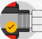
Safety tip: To avoid any wrong connections or air leakage, never mix thread types.
